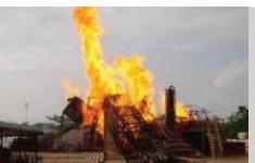
The subject exploration well suffered a blowout and was on fire, while drilling a 12 1/4" hole at a depth of 1704'. The well was flowing gas, believed to be from a charged shallow sand zone. The actual source of the gas was not confirmed, but it was later determined that there was a casing leak on a nearby well located on the same drilling pad. Cudd Well Control (CWC) was contacted to assist in the well control operations.
